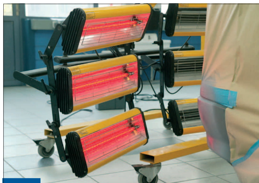
8 Infrared drying topcoat
